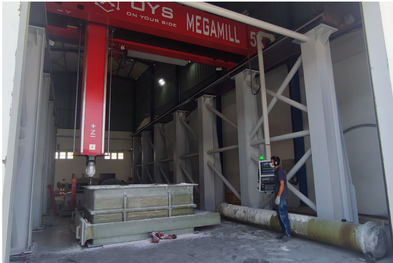
LARGE 5 AXES CNC MACHINE 5m x 15m x 5m
