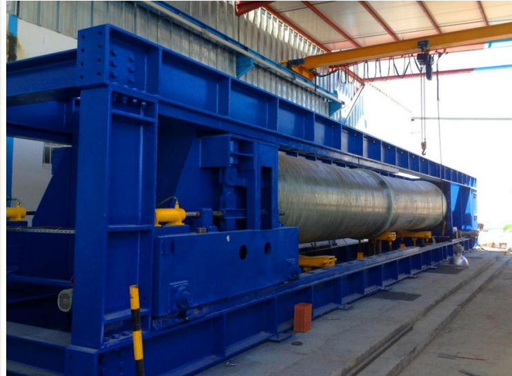
Pressure test for buried pipes
