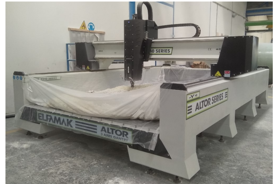
CNC MACHINE FOR GRP 4m x 2m
