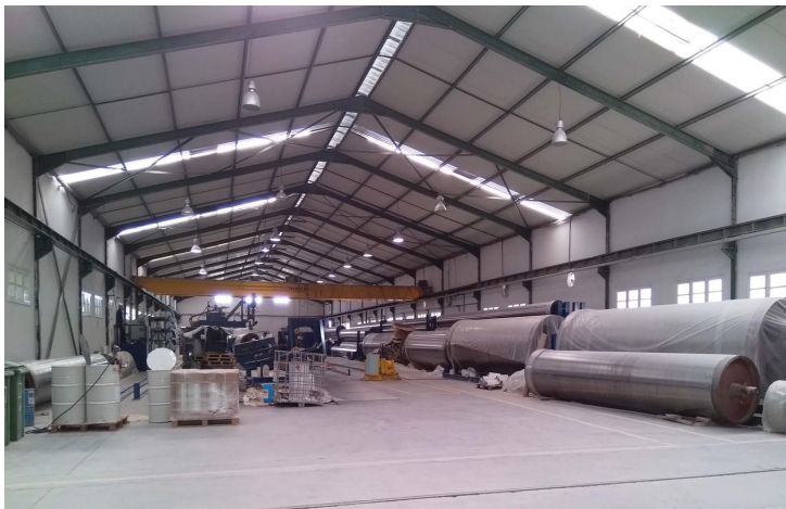
6 filament winding machines DN300 to DN1800
