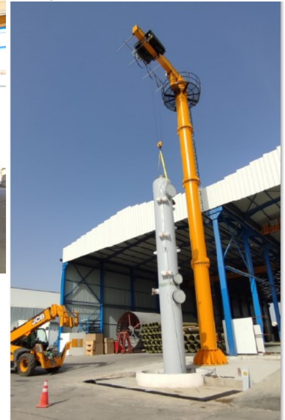
Pressure test of scrubber
