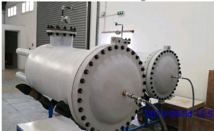
Pressure test of catridge filters
