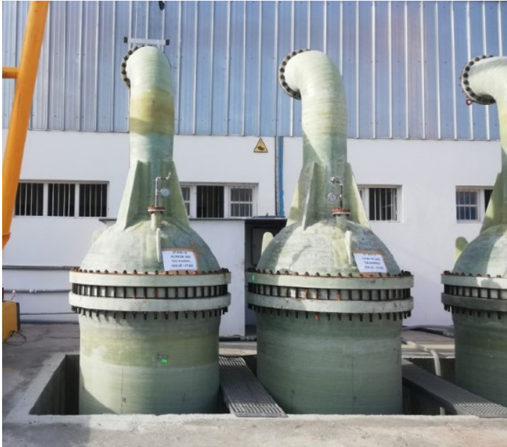
Pressure test of catridge filters
