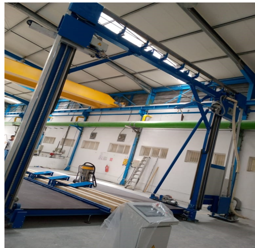
CNC SAW MACHINE UP TO 3500mm
